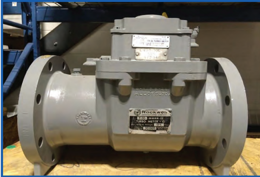
FIGURE 2: Utility-type turbine flowmeter for natural gas custody transfer. Courtesy: Enbridge Gas Distribution Inc.
