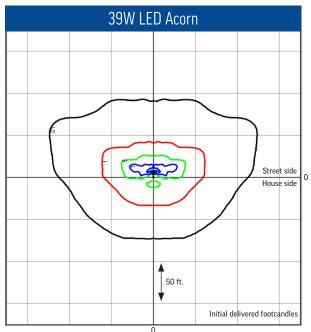
Distribution: type 3 roadway Initial delivered lumens: 5,246 Luminaire mounting height: 13.5 feet
