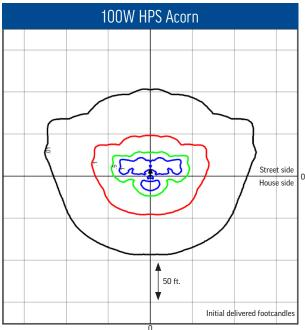
Distribution: type 3 roadway Initial delivered lumens: 9,277 Luminaire mounting height: 13.5 feet
