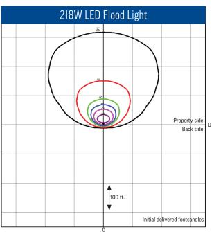
Distribution: 7 H x 6 V NEMA Initial delivered lumens: 29,000 Luminaire mounting height: 26 feet Aiming angle: 60° from horizontal
