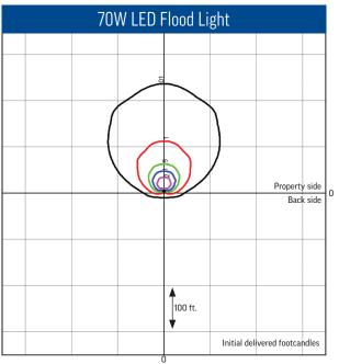
Distribution: 6 H x 6 V NEMA Initial delivered lumens: 9,300 Luminaire mounting height: 26 feet Aiming angle: 60° from horizontal
